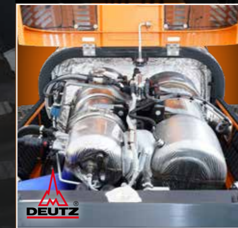
MOTORE DEUTZ DA 100 CV STAGE V DEUTZ ENGINE 100 HP STAGE V
