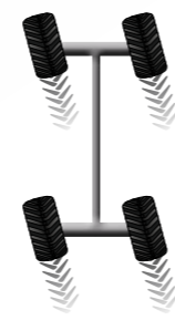
4 RUOTE STERZANTI PARALLELE 4 PARALLEL STEERING WHEELS
