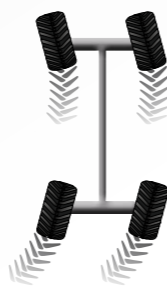
4 RUOTE STERZANTI IN TONDO 4-WHEEL STEERING
