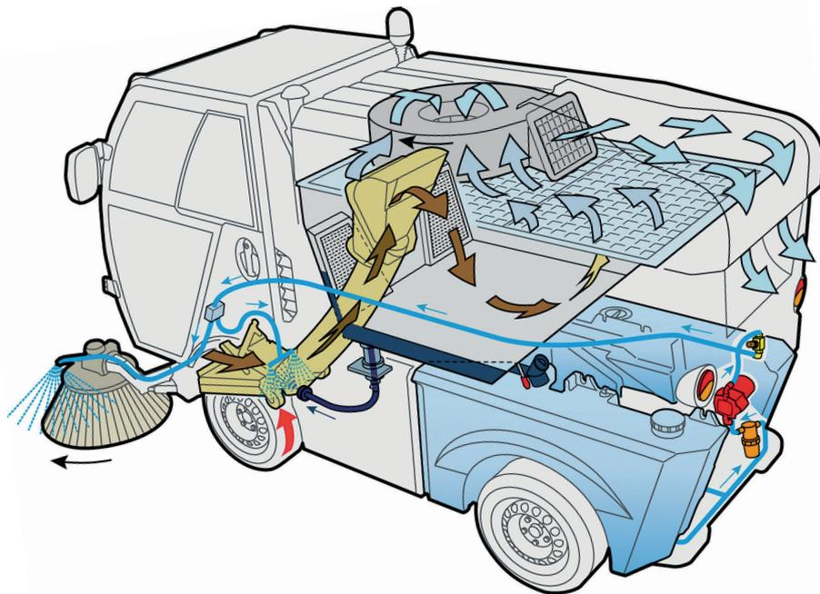
The diagram shows the flow of air from the suction nozzle through the hopper and out through the exhaust duct on the hopper roof. A water pump feeds fresh water to the spray jets fitted to the sweeping brushes and the suction nozzle. The used water is filtered and then fed to the suction nozzle to ensure optimum dust suppression.
