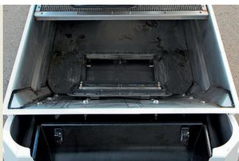
**Hopper with water recirculation** The stainless steel hopper has the largest capacity in its class. The water recirculation system results in drier loads and extends service times.
