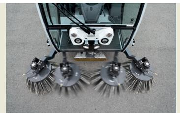
**Impact-protected brushes** The brushes can be extended individually on both sides with stepless adjustment. Brush pressure is fully adjustable and controlled from the driver's cab.
