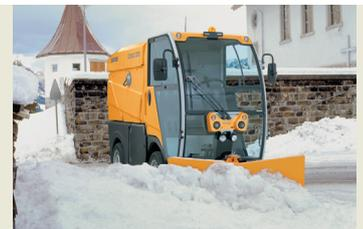
**Snow plough and salt spreader** The snow plough is used to clear snow from roads and footpaths. The salt spreader can be operated at the same time to provide a full, cost-effective winter service.
