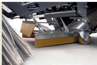
**Impact-protected suction nozzle** Supported by castor wheels, the suction nozzle is located between the front wheels and fitted with water spray jets. A special mounting allows it to ride over obstacles without damage to the nozzle.
