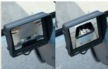
**Suction nozzle and reversing camera system** The reversing camera provides improved visibility and reduces the risk of collision with obstacles or other road users during daily operation. The suction nozzle camera enables improved inspection of the suction nozzle intake.
