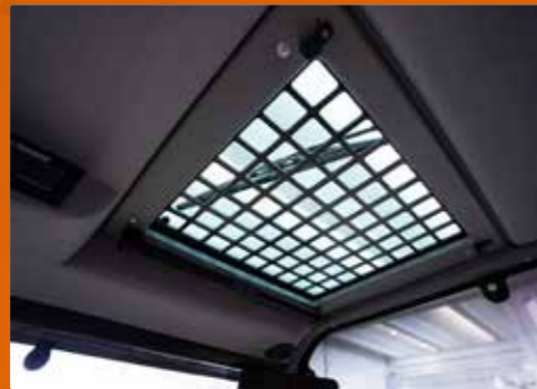
Oblò in cabina (Solo con cabina PRESTIGE) Cabin porthole (Only with PRESTIGE cabin)
